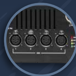
4 DMX outputs to expand DMX outputs from the console
